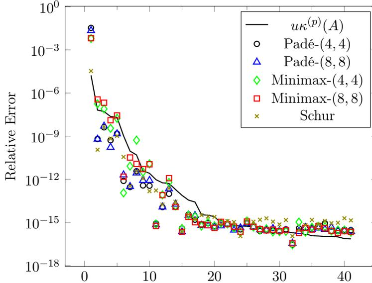
Figure 5: Relative errors committed by the Padé iterations of type (4, 4) and (8, 8), the minimax iterations of type (4, 4) and (8, 8), and the Schur method [30]. Results are shown for 41 tests with  $p = 3$ , ordered by decreasing condition number  $\kappa^{(p)}(A)$ .
