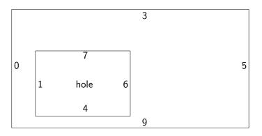
We can discretize the "plate" into discrete points and transform the PDE into a linear system to be solved, iteratively.
